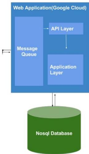
Web Application consists of the Message Queue. For the Smart Watering Application, we have used Pubnub message queue for the application messaging.
