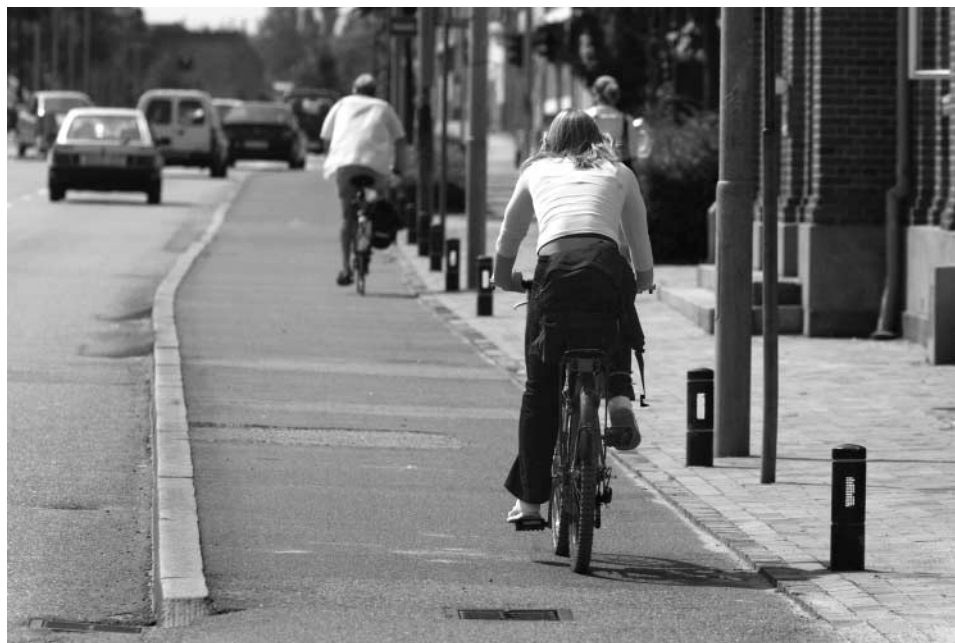
Figure 16. Green wave for cyclists in Odense, Denmark. Bright green lights on the bollards along the path pulsate in a wave-like forward motion guiding cyclists to the next green traffic signal at 20km/hr. If cyclists keep pace with the green wave, they get green traffic signals at all intersections.
